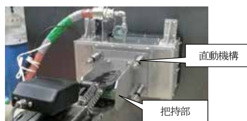
写真9 低所壁面除染治具外観
